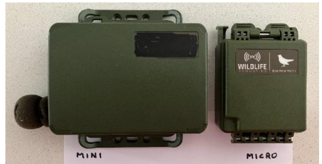
The Wildlife Acoustics Mini and Micro Song Meters and (below) Ken attaching a Mini to a tree where it was left recording for up to five days
