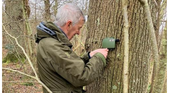
The Wildlife Acoustics Mini and Micro Song Meters and (below) Ken attaching a Mini to a tree where it was left recording for up to five days
